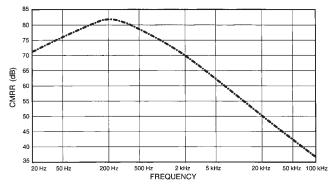
Typical CMRR: From 20 Hz to 100 kHz with input voltage of 6 volts.
